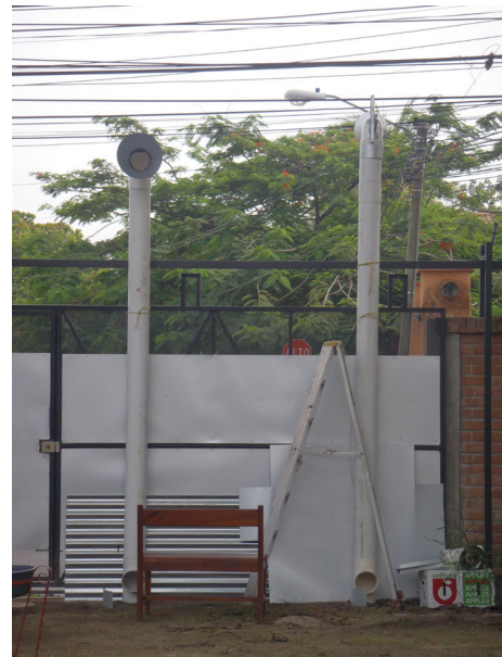
Figure 20 Set up with leeward and windward facing pipe.
